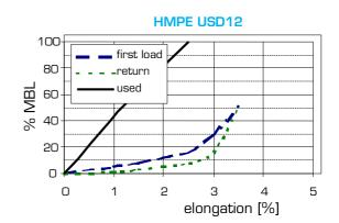
MBL = Minimum Breaking Load conform ISO 2307
