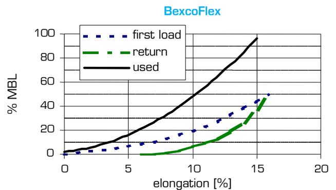
MBL = **M**inimum **B**reaking Load conform ISO 2307
