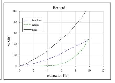
MBL = Minimum Breaking Load conform ISO 2307
